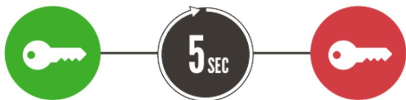
**Option B:** Turn the ignition on, then off to wake the RIDE Core. Arm Transport Mode from the app. The device can now be unplugged without triggering the back up battery.
