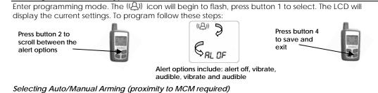
Enter the programming mode. Scroll to the **b** icon and press button 1 to enter the arming selection screen. The LCD will display the current setting (**[Act]** or **[PAS]**) and the siren will chirp two or three times. To program follow these steps:
